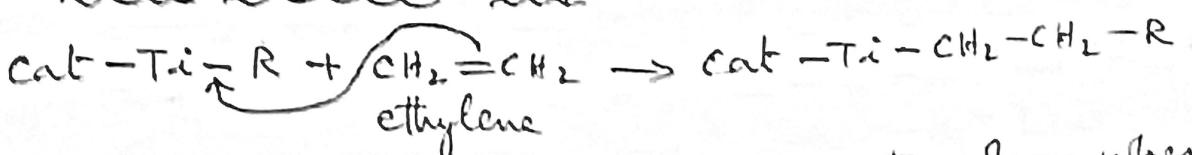
This Ti-C bond is the active centre from where the propagation starts.
