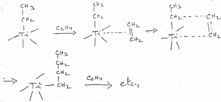
The stereospecific and stereoregular polymers are obtained. Because of non-equivalence of the coordination sites of olefin and active alkyl group at the active titanium center, the growing alkyl gp moves back to its original position after each insertion of a new monomer.
